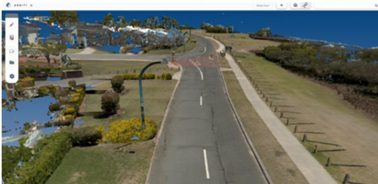
Figure 3.6: Coloured LiDAR Point Cloud, generated through mobile LiDAR and 360-degree imaging
