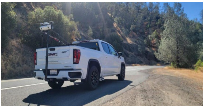
Figure 3.4: Initial profiler and sample output (a) Inertial profiler from SSI, (b) Point cloud of a highway section
