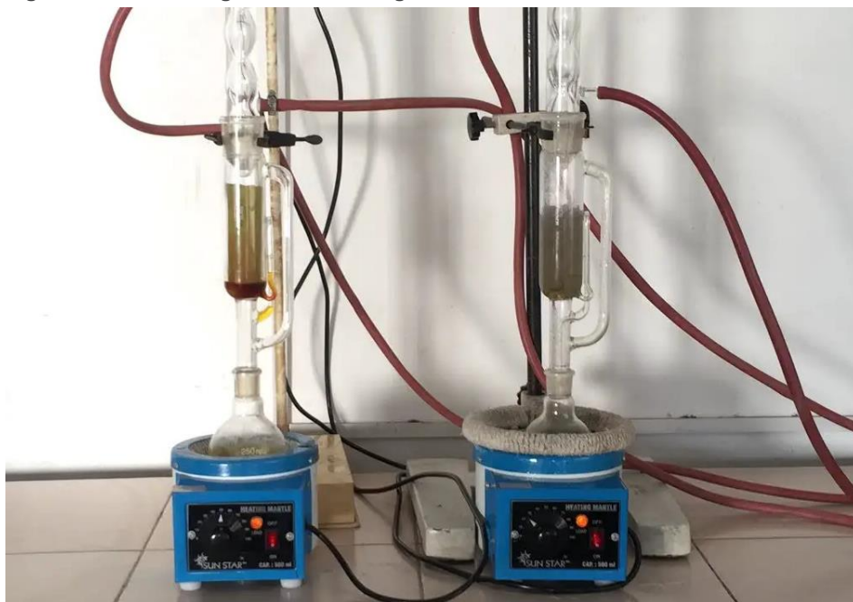
Figure 3.3: Washing of CRMBs using a Soxhlet extractor
