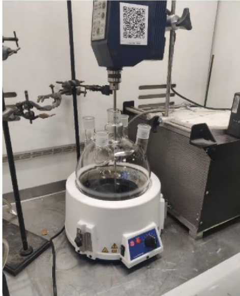
Figure 2 – Setup of fume generation chamber inside fume cupboard
