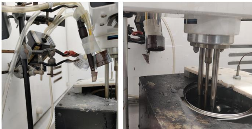
Figure 3.11: Placement of static samplers during binder blending
