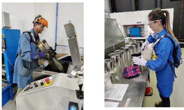
Figure 1 – Laboratory staff members wearing backpack with sampling pumps and devices during asphalt testing.
