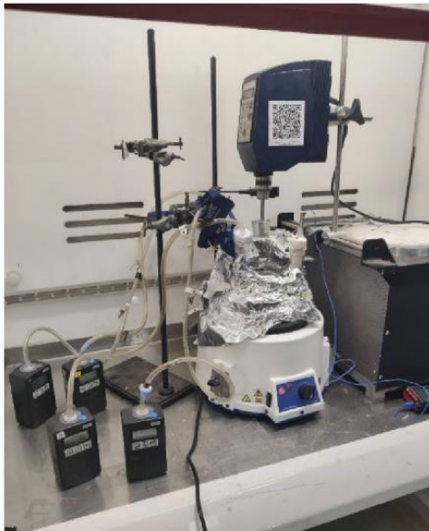
Figure 3 – Setup of headspace sampling emission train
