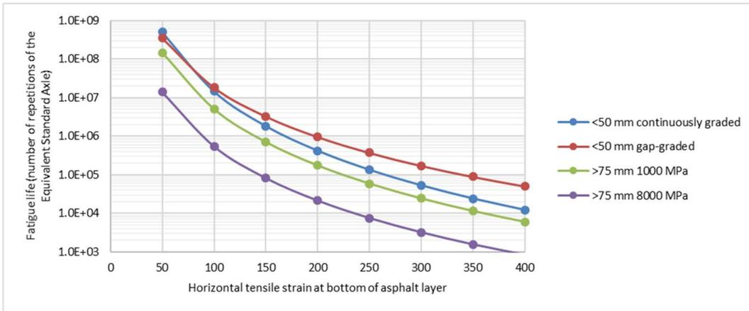
Figure C 7: South African asphalt fatigue transfer functions for a reliability level of 95% with shift factor
