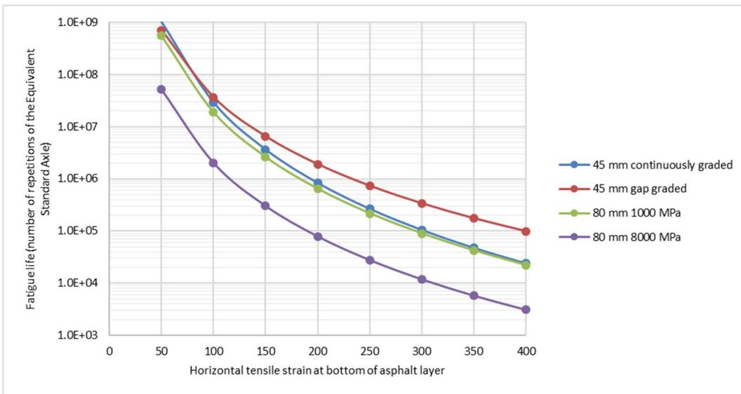
Figure C 8: South African asphalt fatigue transfer functions for a reliability level of 95% with shift factor compared to Austroads (2018)
