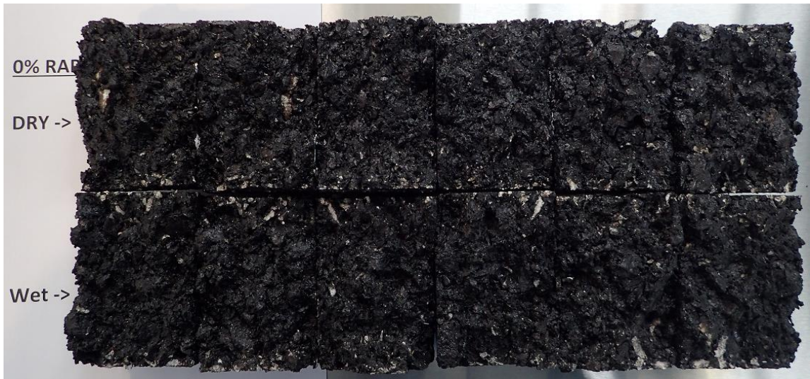
Figure 6.2: Visual assessment of the degree of stripping of three mixes
