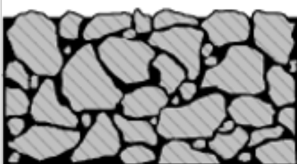
Figure 2.5 Typical gap-graded asphalt mix
