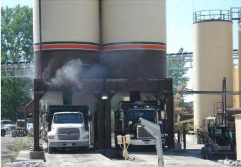
Figure 4.11: HMA fuming (left)/WMA no fuming (right)
