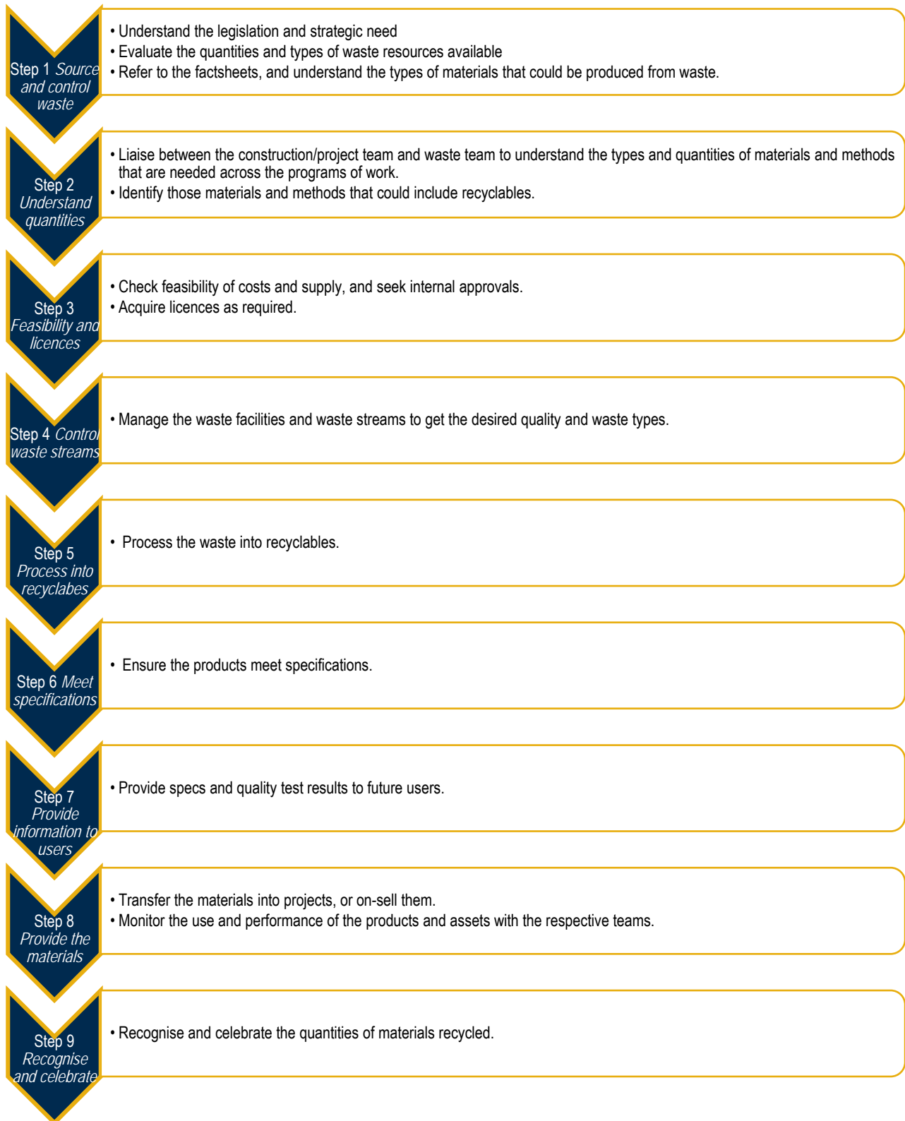
Figure 7.2: The process for managing waste to produce recycled materials for local government projects
