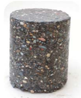
Bitumen emulsion stabilised basecourse with recycled aggregate
