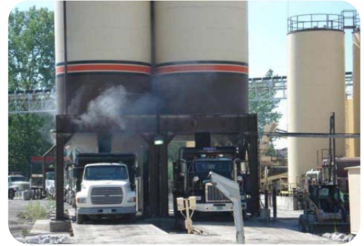
HMA fuming left vs WMA no fuming right
