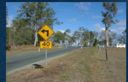
Warning signs Source: ARRB Group.
