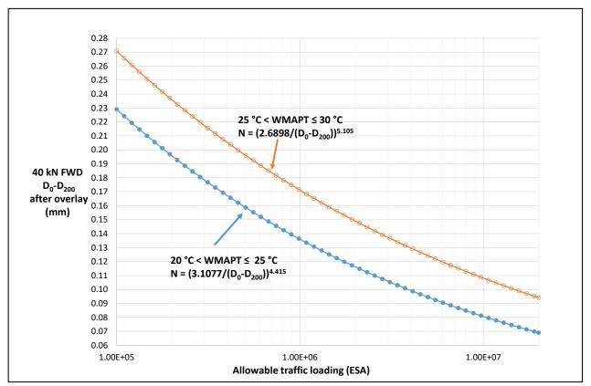
Figure 3.4: 40 kN FWD design curvatures for 50 mm thick asphalt overlay for WMAPTs of 20–30 °C
