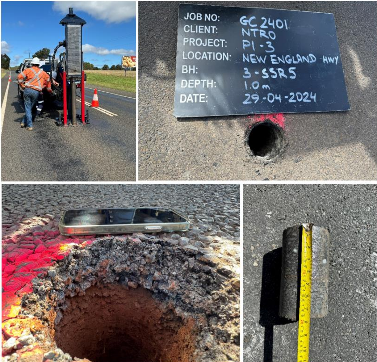
Figure 3.16 Coring and boring and documenting the samples for third round of data collection
