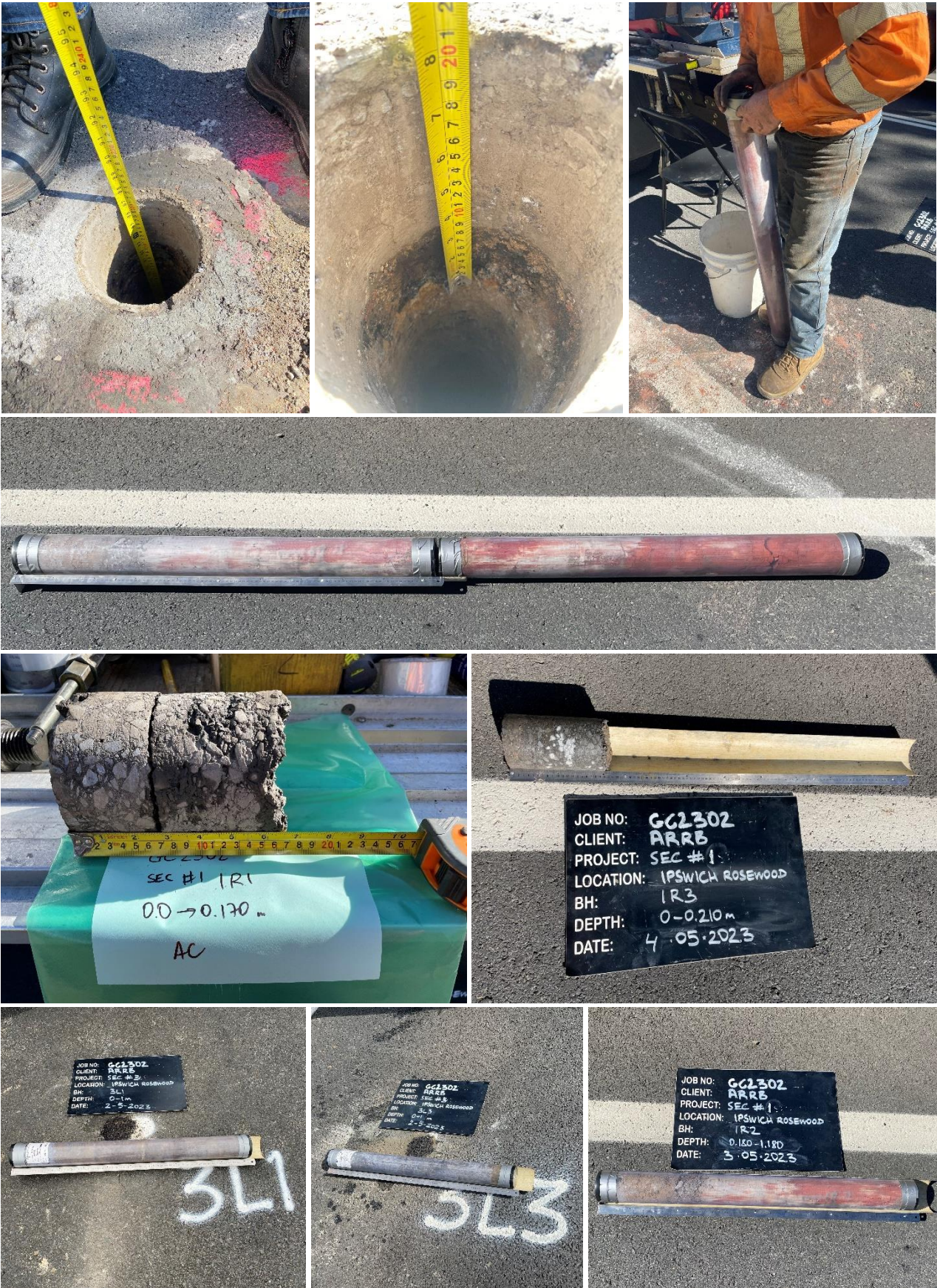
Figure 3.10 Sampling (depth of 1m & 2m), packing the pushed tubes and documenting the samples
