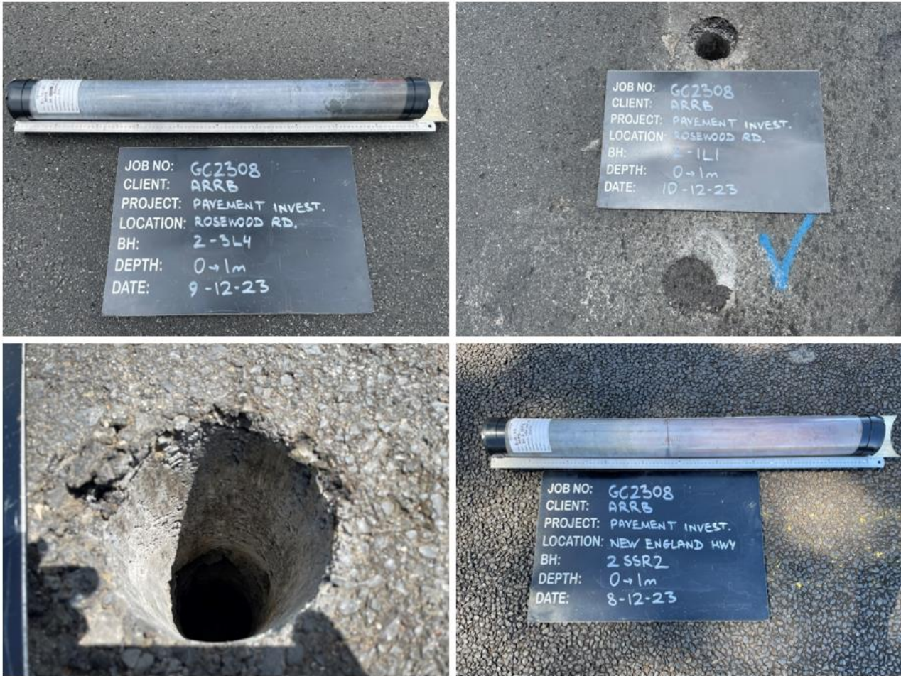
Figure 3.15 Coring and boring and documenting the samples for second round of data collection
