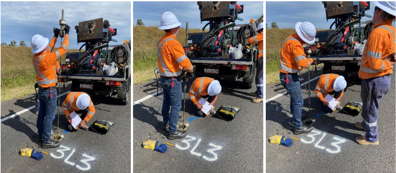
Figure 3.11 DCP test on each test point
