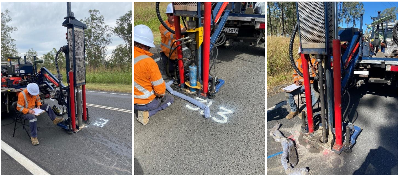
Figure 3.9 Push tube sampling through hammering and core sampling with diamond coring
