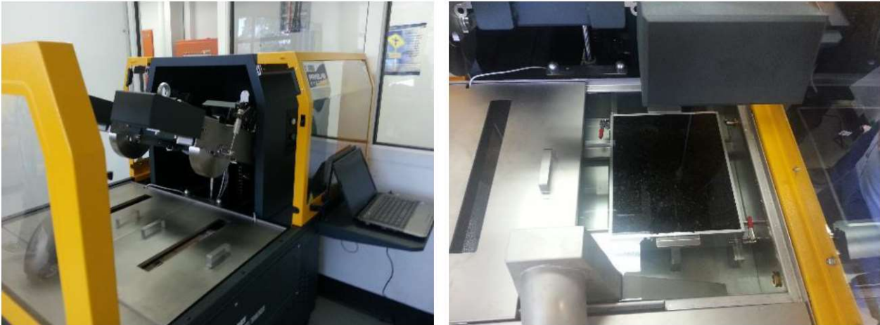
Figure 8.14: HWTD with sample covers (left) and with sample loaded (right)
