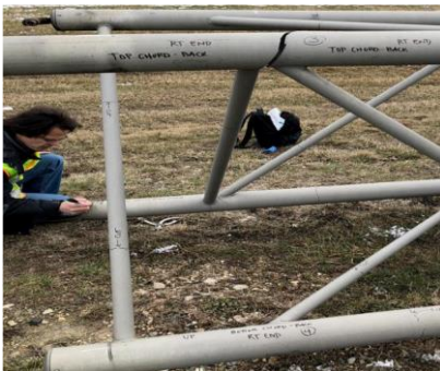
Figure 2.9: Failure of cantilever truss members
