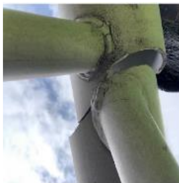
b. Close-up of fracture of chord
