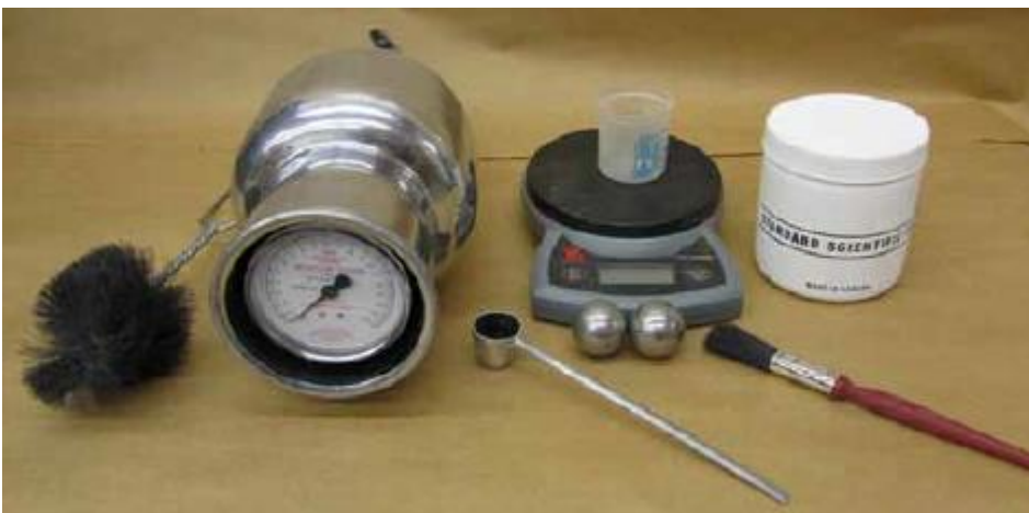
Figure 3.4: Speedy moisture tester
