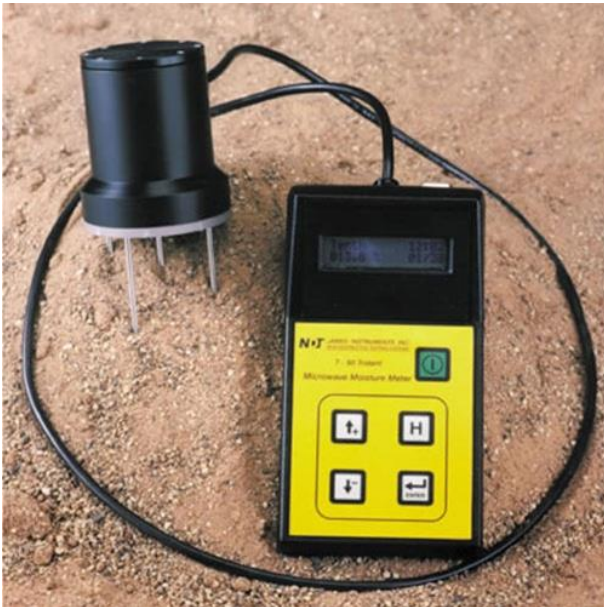
Figure 3.3: Trident moisture meter
