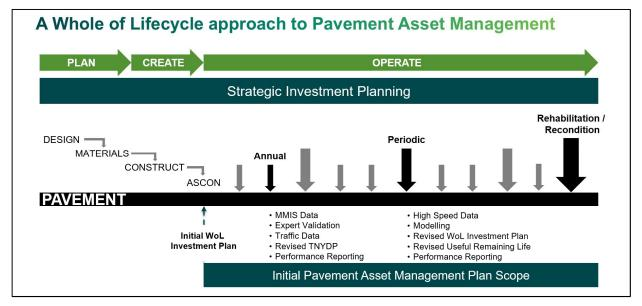
Figure 5.5: A Whole of Lifecycle approach to Surfacing Asset Management
