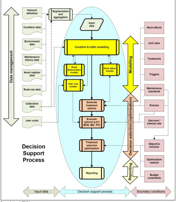
Figure 4.1: Central role of modelling in a pavement management system
