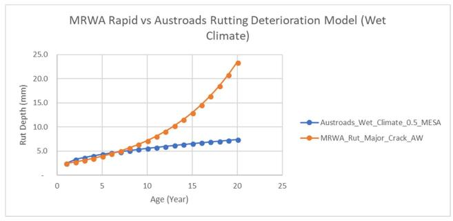
Figure 4.6: Comparison of the Main Roads model estimates and the Austroads rutting models for the rapid deterioration phase
