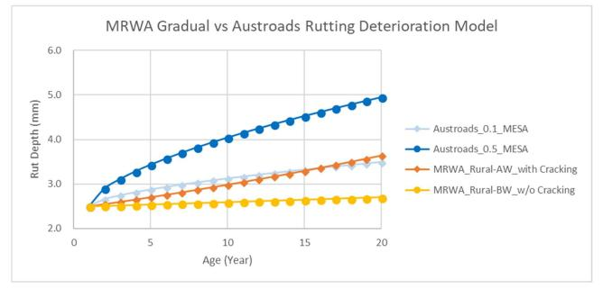
Figure 4.5: Main Roads Gradual versus the Austroads Rutting Deterioration Model
