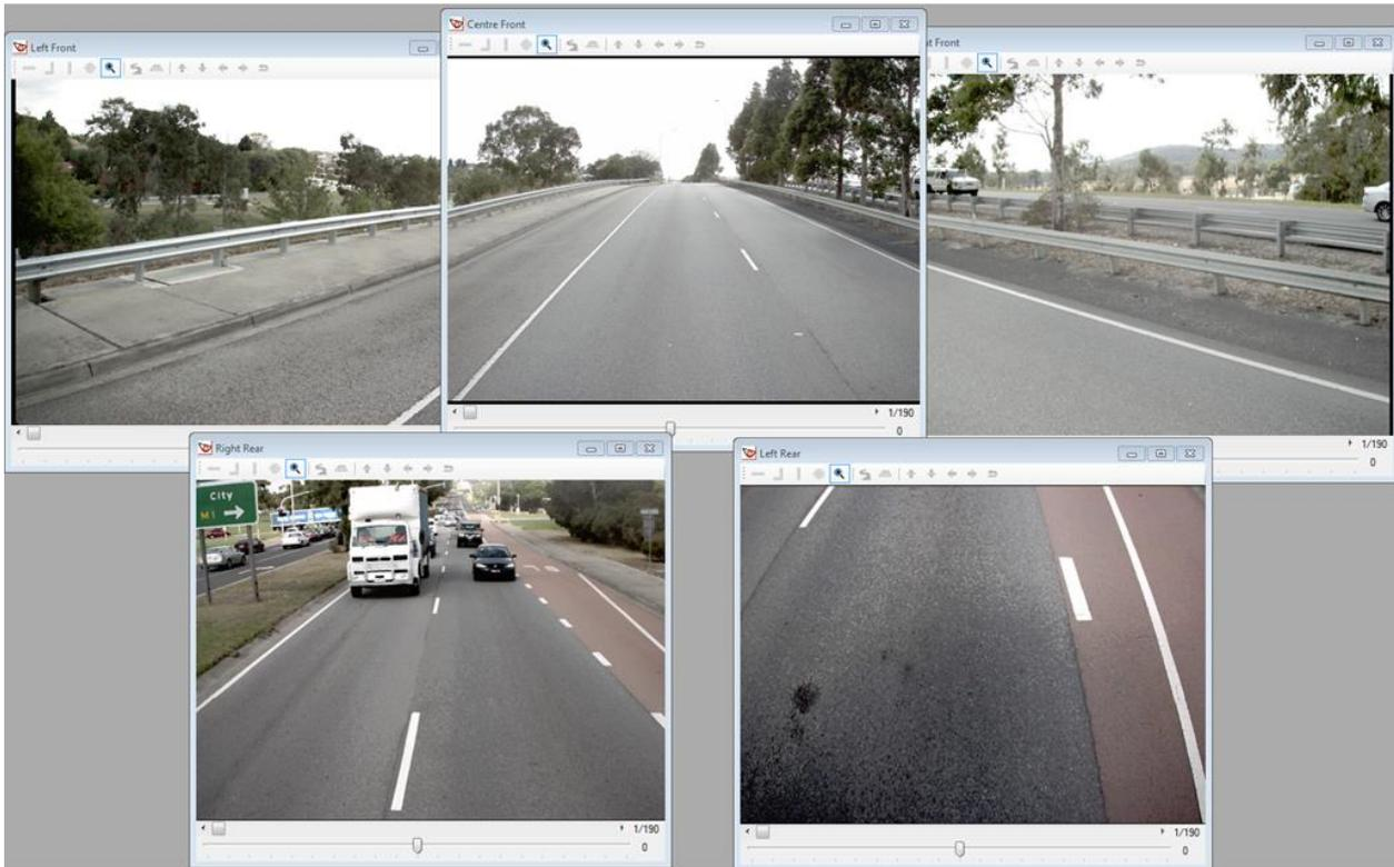
Captured images are referenced by linear position (in relation to road location information) and geospatially (latitude and longitude). This makes it possible to locate defects or features on the network by chainage and spatial coordinates. This facility also makes it possible to capture inventory information, complete with a unique GPS position.
