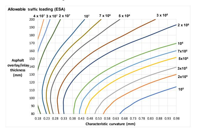
overlay / inlay thicknesses of 80 - 200 mm
