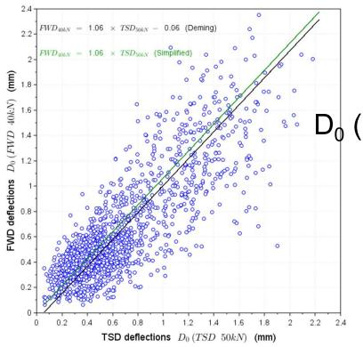
$D_0^{\perp}$  (FWD 40 kN) = 1.06  $D_0^{\perp}$  (TSD 50 kN)
