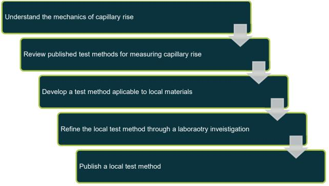
This project undertook a vast review of national and international literature as a first step followed by design and execution of an in-depth laboratory investigation. The laboratory investigation included development of a suitable sample apparatus, specification of sample preparation steps and test duration in addition to detailing the required calculations and measurements for obtaining a capillary rise height.
