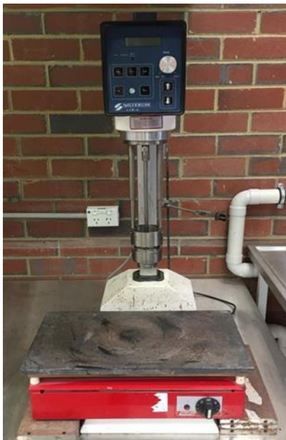
Figure 12.1: Silverson high-shear mixer
