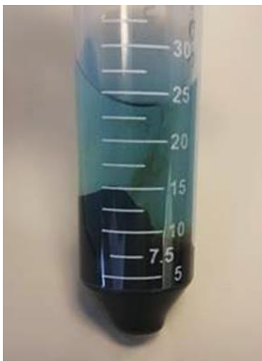
Figure 12.6: Virgin bitumen (75 mg) in commercial kerosene at 25 °C (t = 0.0 min.)
