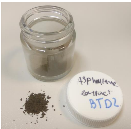
Figure 12.17: Asphaltene particles with NS particles
