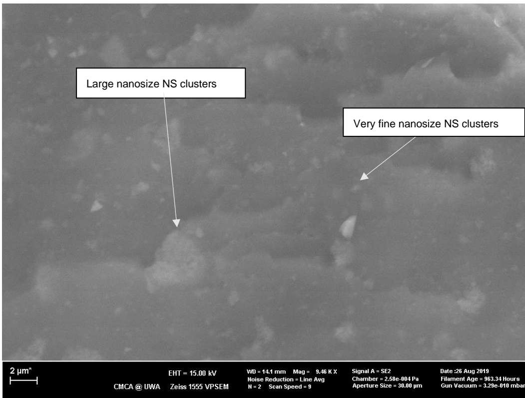
Figure F 30: SE image – frozen unaged C320 + 6% NS (20nm + KH550 Couplant)
