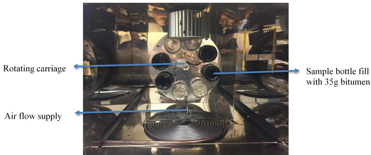
Figure 12.11: Rotating bottle carriage of RTFO
