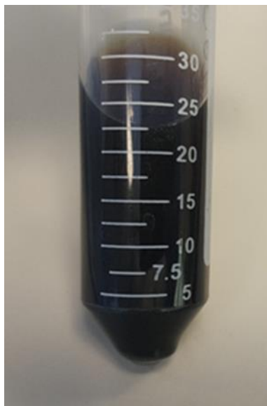
Figure 12.7: Complete dissolution of virgin bitumen in commercial kerosene at 25 °C (t = 12.0 min.)
