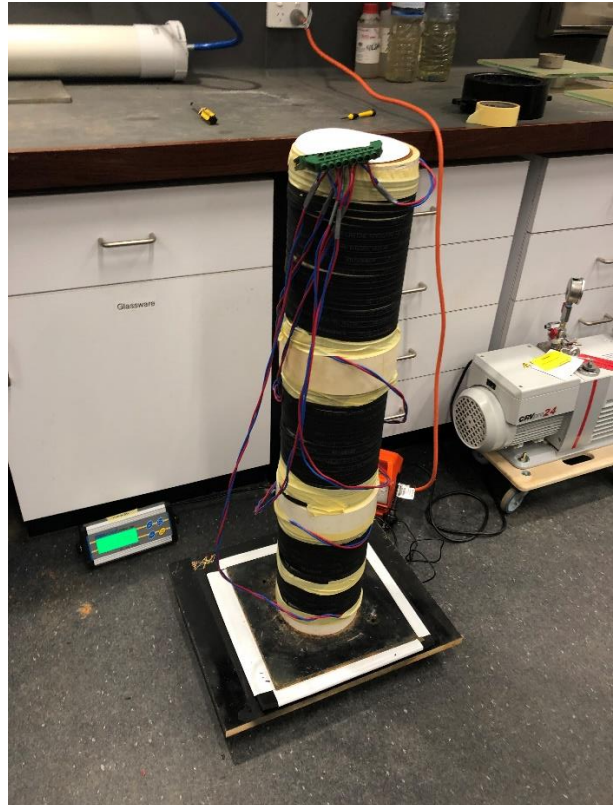
Figure 6.3 Moulded sample wrapped with heat tape
