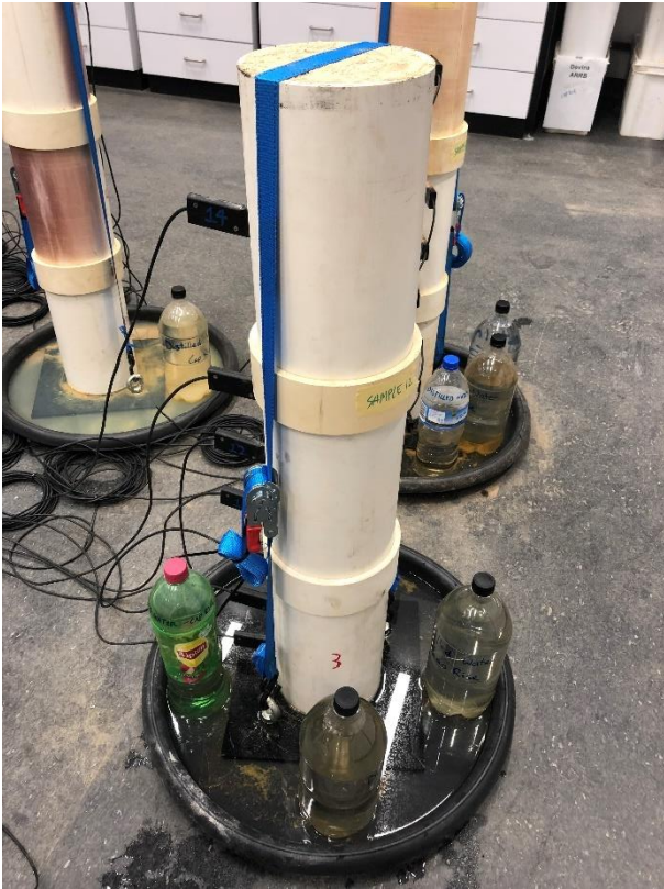
Figure 6.4 Sample set-up with constant head water bath
