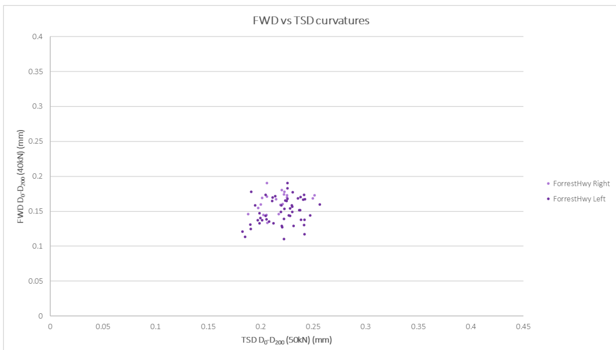
Figure D.4 Visual inspection of FWD vs TSD curvature ( D_0 - D_{200} ) – Forrest Highway
