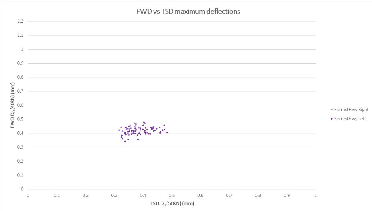
Figure D.3 Visual inspection of FWD vs TSD maximum deflections ( D_0 ) – Forrest Highway
