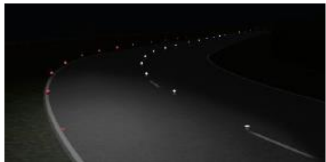
Figure 2.19: Simulator retroreflective/solar road stud on rural road
