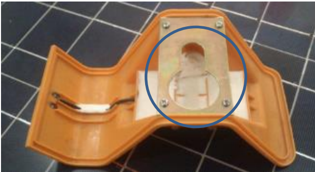
Figure 2.29: Hybrid retroreflective/solar LED guardrail markers
