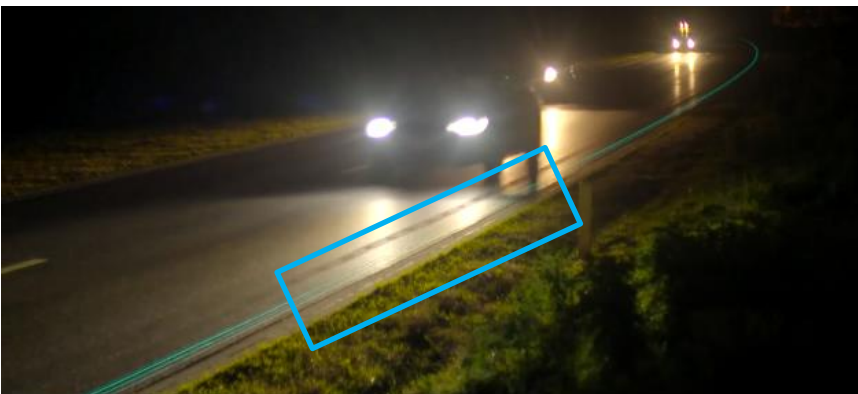
Figure 2.6: Headlights overpowering luminescent line marking
