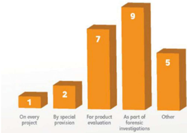
Figure 6.2: When US agencies perform interface bond testing
