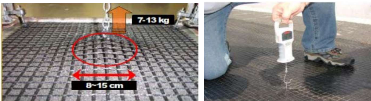
Figure 2.1: Spring balance testing
