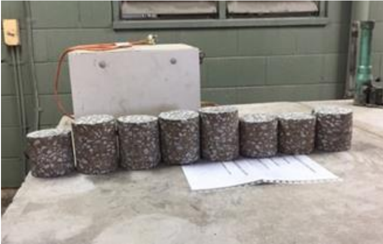
Figure 5.6: EME2 sample cores at Boral laboratory for density testing
