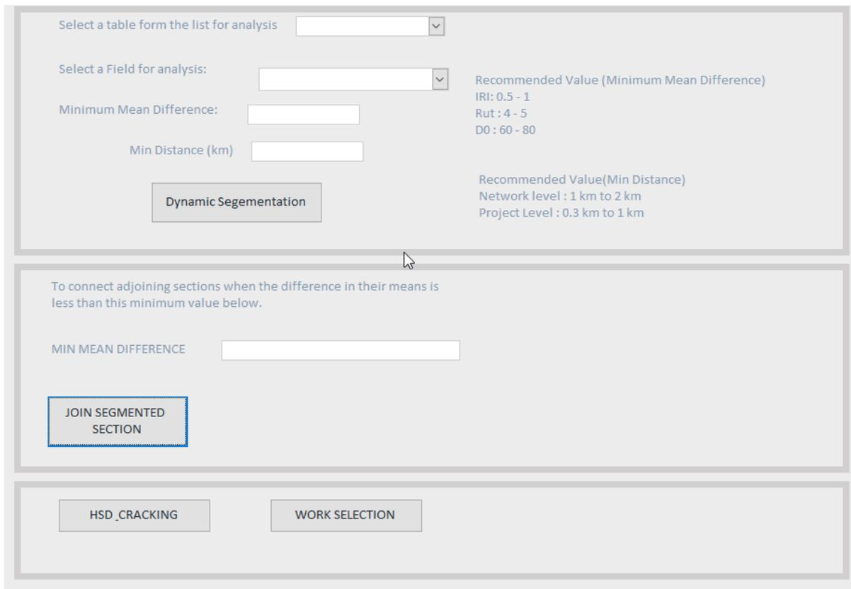
After segmenting the road based on deflection ( $D_0$ ), the HSD\_CRACKING button can be used to average other road performance measures (roughness, rutting, texture and cracking) into one table. This table can later be used to aid work selection. This table contains basic road information such as LINK\_ID, Dist\_from, Dist\_to, etc. and thus can potentially be linked directly with MRWA pavement management system output.
