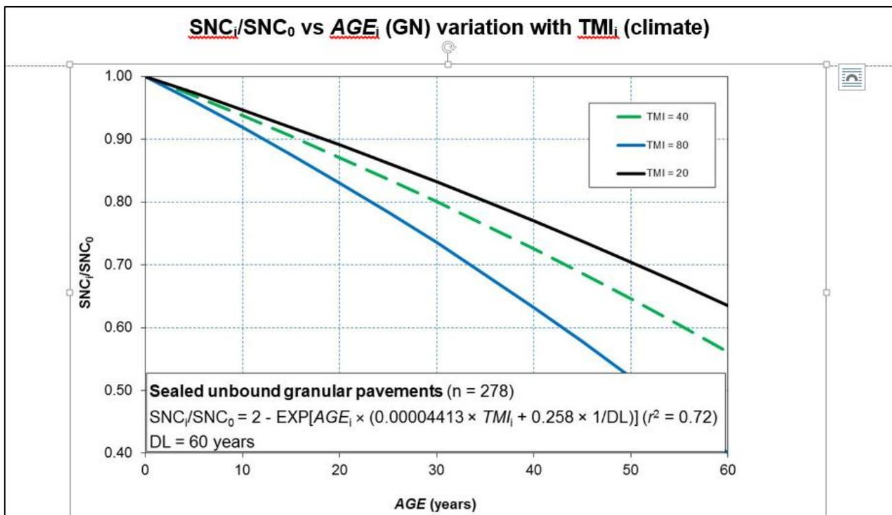
The current strength of the pavement is defined in terms of the SNC at the time of the most recent structural testing (time 'i'), calculated based on the measured peak deflection ( $D_0$ ) under loading. It involved calculating  $SNC_i$  firstly by converting TSD outputs to FWD values as detailed in Section 2.2, and then converting these to equivalent Benkelman beam ( $D_{0-BB}$ ) values, and finally applying Equation 6 and Equation 7 from Patterson (1987).
