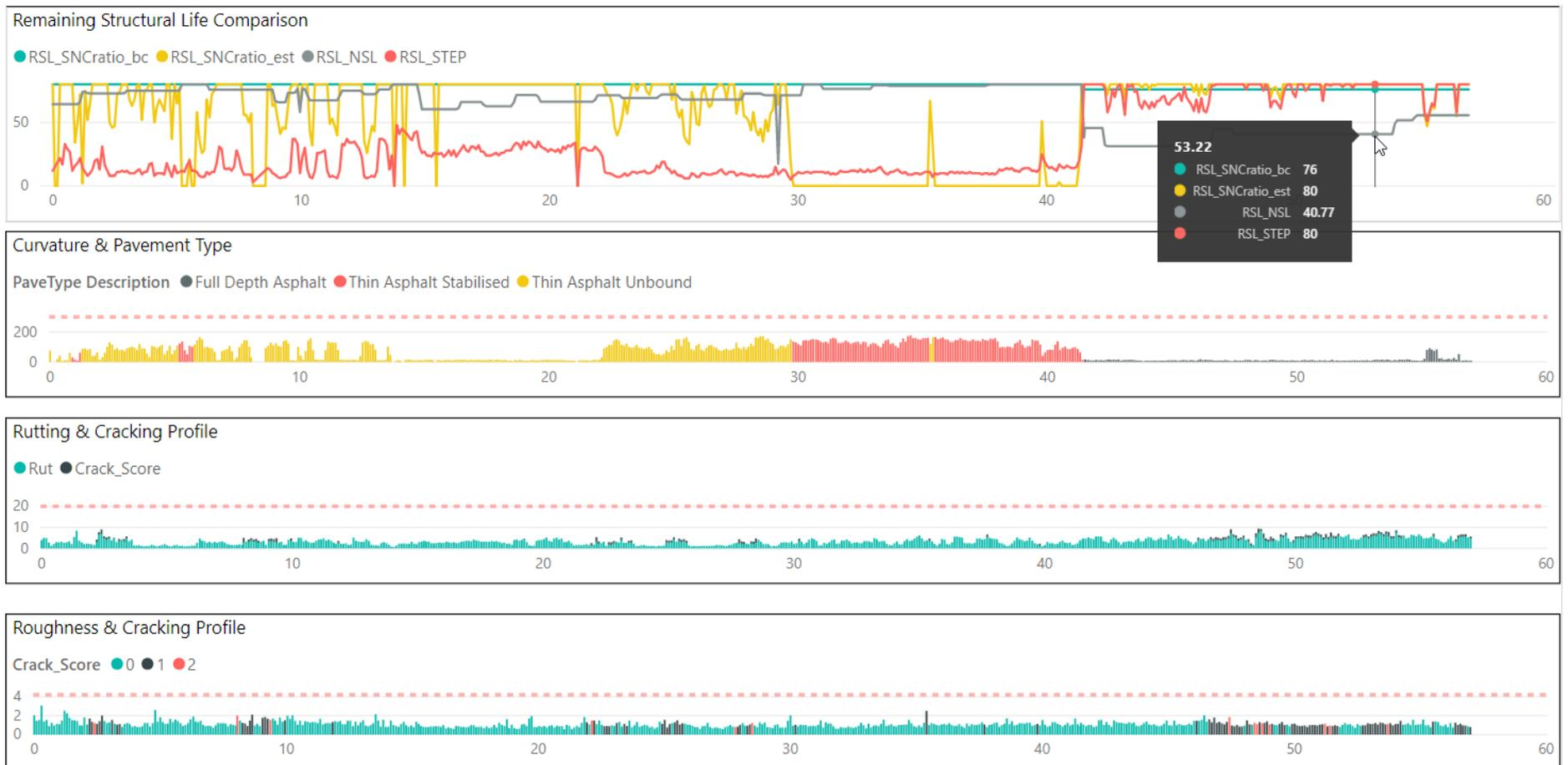
Figure 3.8: Great Eastern Highway (H005) Structural Capacity Comparison
