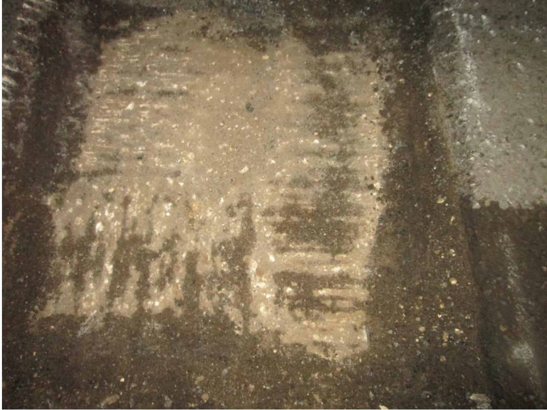
Figure A 4: T4 granular profile and subgrade surface
