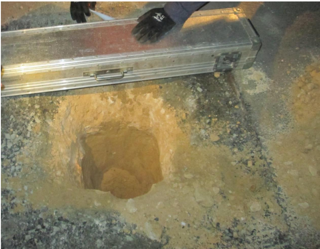
Figure A 4: T4 granular profile and subgrade surface
