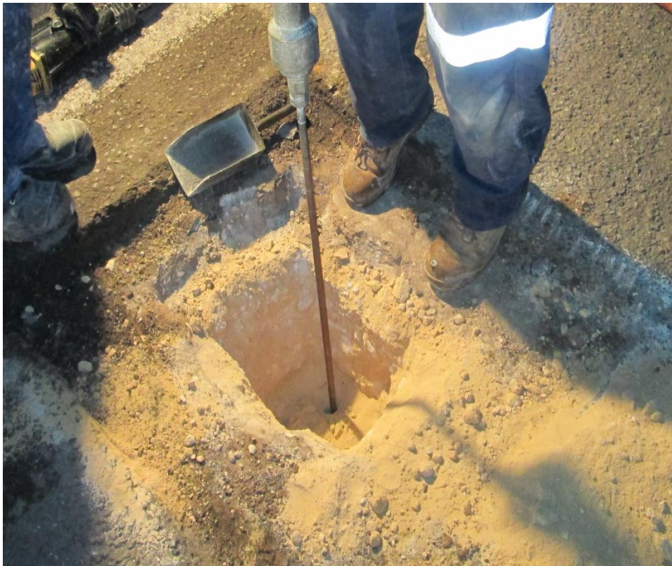
Figure A 2: T2 granular profile and subgrade surface
