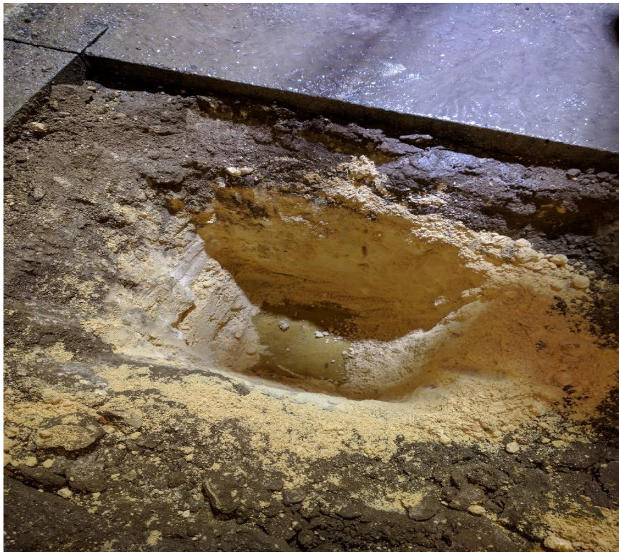
Figure B 2: R2 granular profile and subgrade surface
