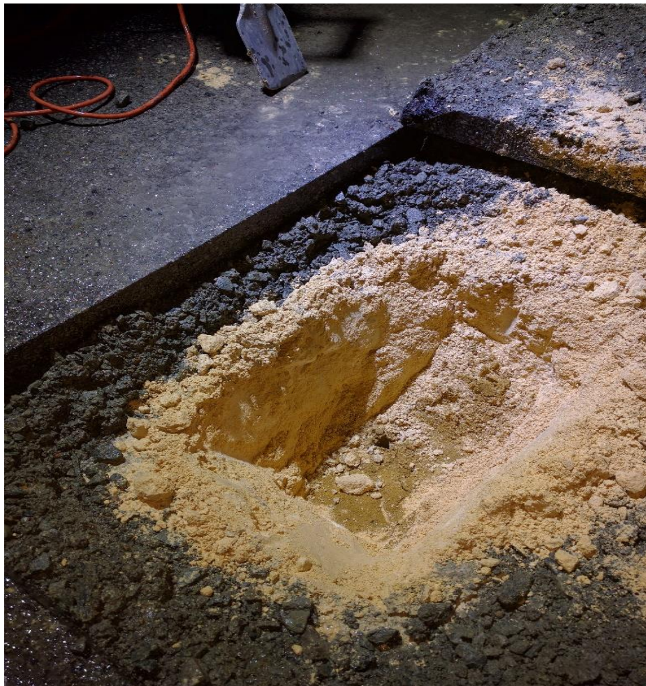
Figure B 4: R3 granular profile and subgrade surface
