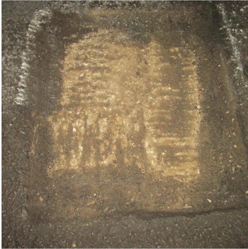
Figure A 2: T2 granular profile and subgrade surface
