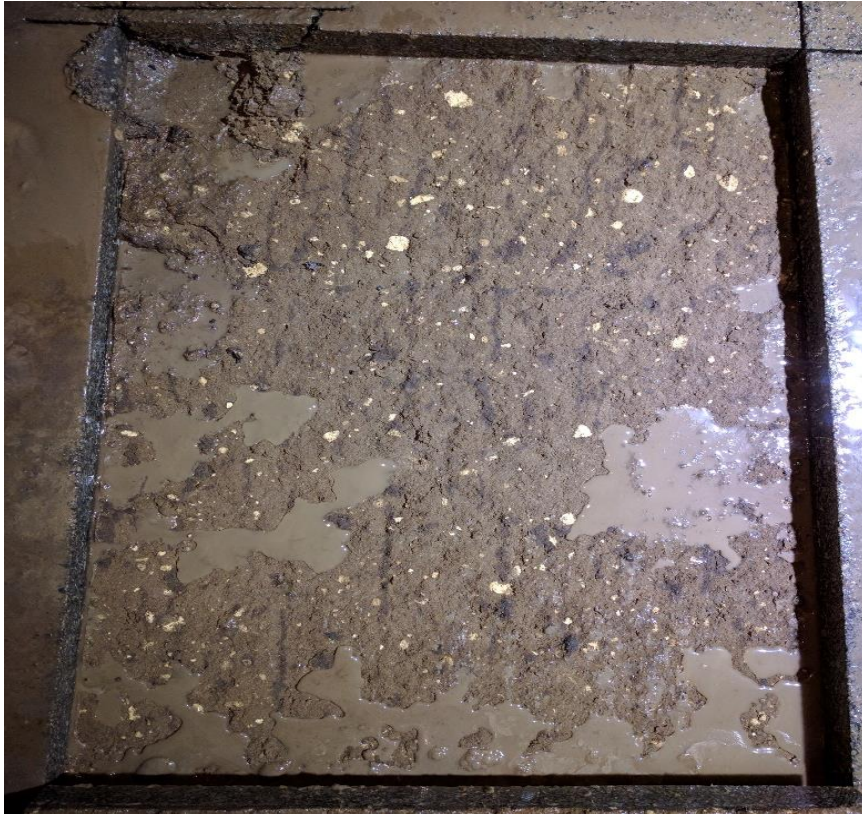
Figure B 2: R2 granular profile and subgrade surface
