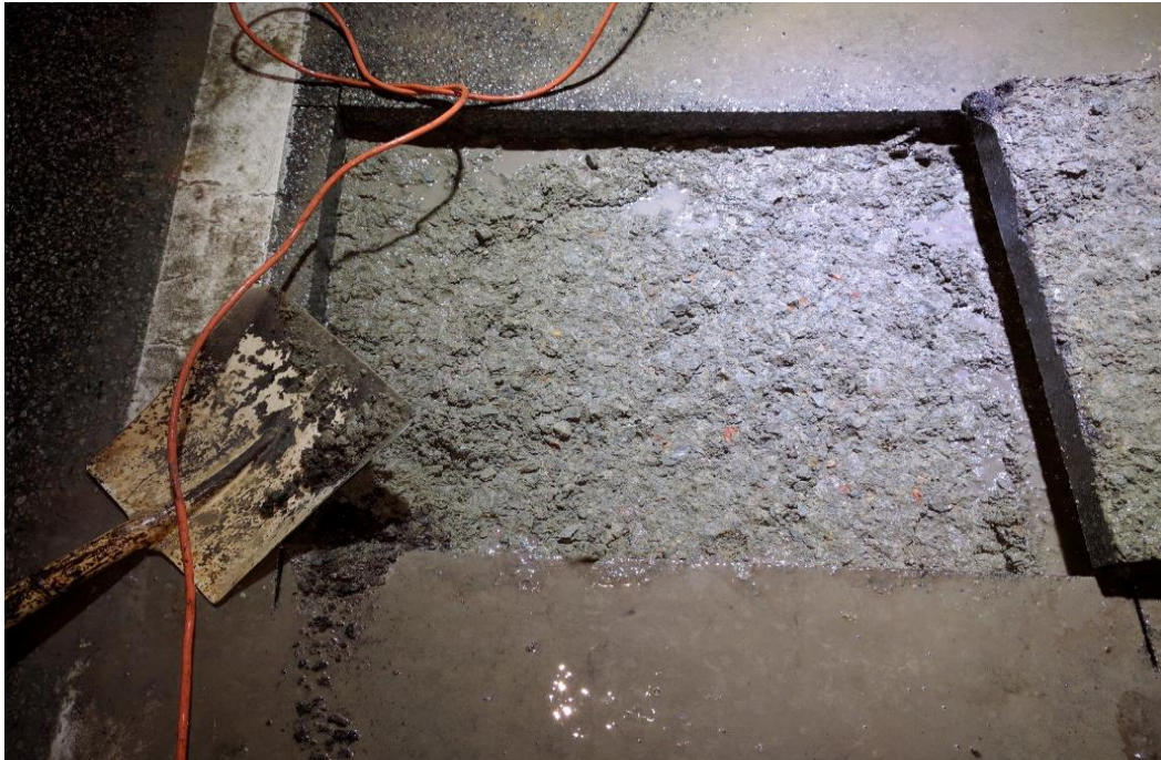
Figure B 4: R3 granular profile and subgrade surface
