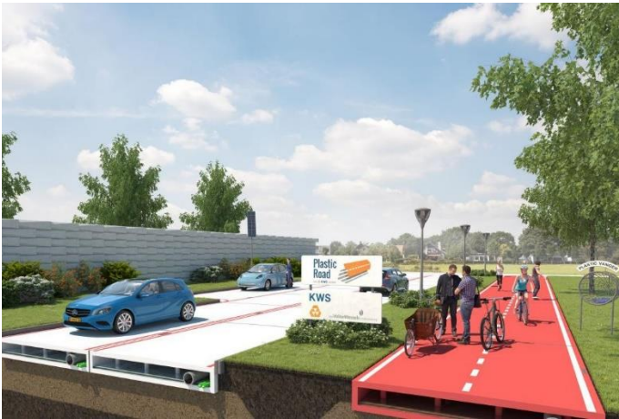
Figure 3.4: Conceptual model of Dutch modular pavement system
