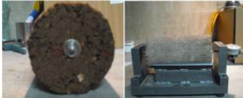
Figure 6.1: Shrinkage measurement of crushed recycled concrete
