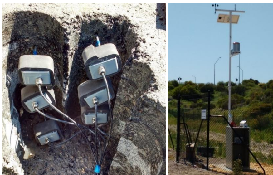
Figure 2: Pavement temperature sensors and weather station at Jandakot
